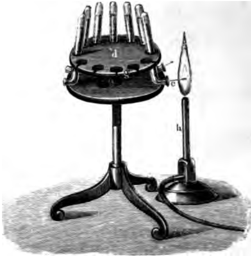
FIG. 67. --Mitscherlich's arrangement for flame spectra. c, wick ; A, Bunsen's burner.
